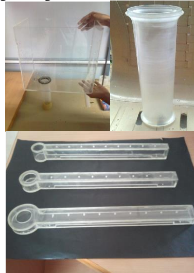
Figure 2. Fabricated pouring basin with sprue and runner models signifying three different aspect ratios
