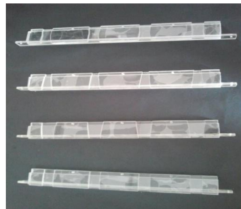
Figure 2. Fabricated pouring basin with sprue and runner models signifying three different aspect ratios
