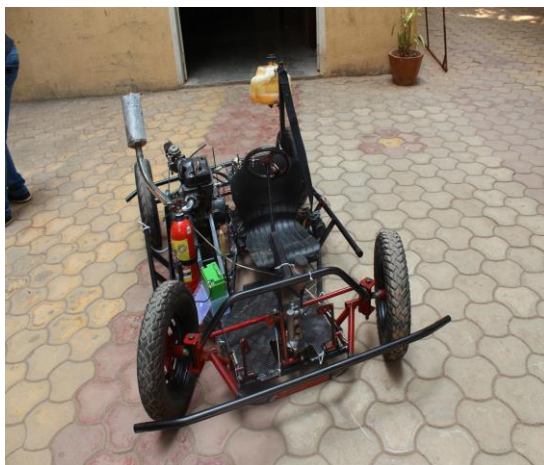
Fig.11. Steering System manufactured and mounted on the vehicle.
