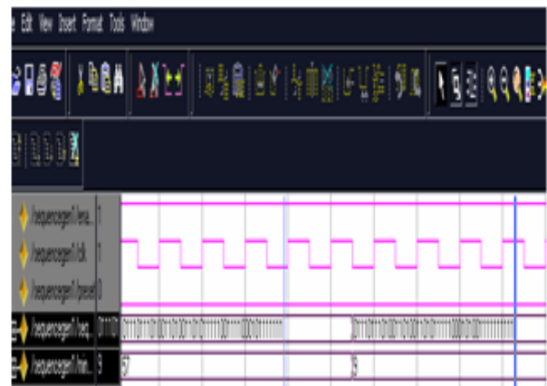
Fig. 2 Behavioral simulation result of a good 23-bit Binary Pulse compression sequence.
