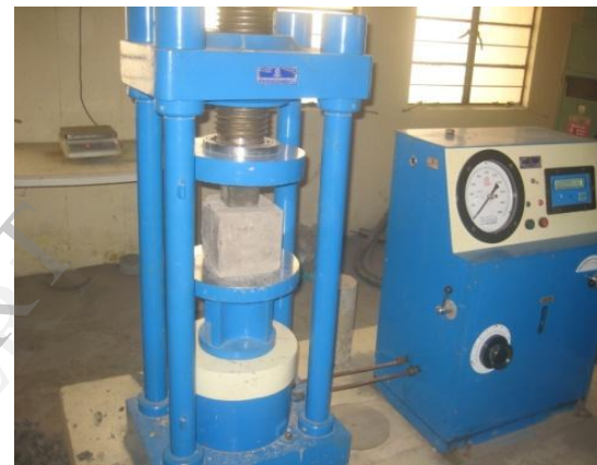
Fig9: compressive strength of cement testing setup
