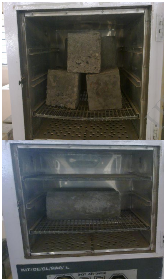
Fig5: Hot curing of specimens
