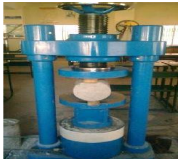
Fig16: split tensile testing setup
