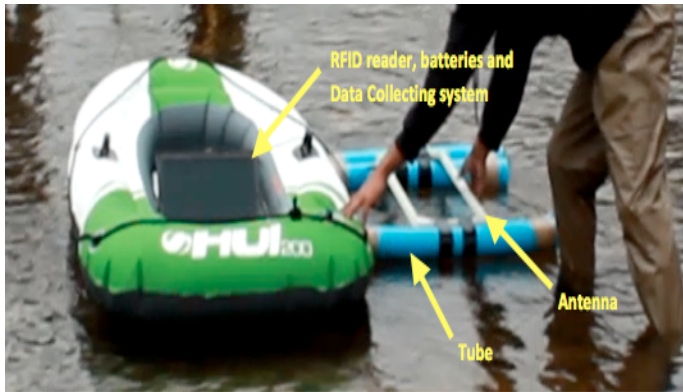
Fig. 2 Installing the RFID system near bridge pier
