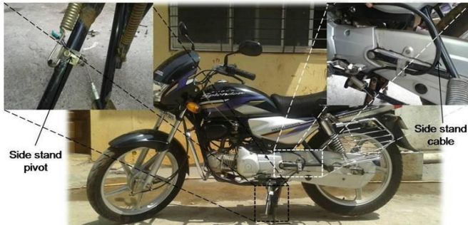
Fig. 6 a. proposed system mounted on two wheeler showing side stand pivot and side stand cable
