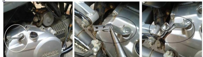
Fig. 4 Mounting of clutch shifter lever
