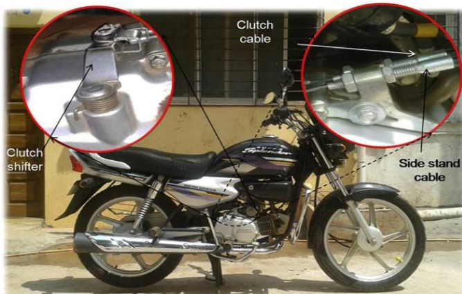
Fig. 6 b. proposed system mounted on two wheeler showing clutch shifter and both cables
