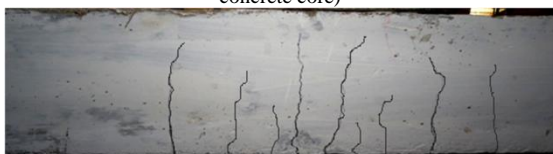
Fig 10.2 BEAM - Hdc2 (Double layered Hexagonal wire mesh with concrete core)
