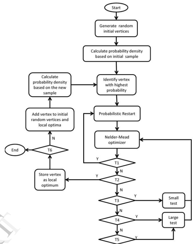
Figure 1: GBNM restarts schematics. T1: (this point is already known as a local optimum). T2: (vertex ix a local optimum). T3: (large test or probabilistic and not return to the same point and point on the bound). T4: (small test and not return to the same point and not on the bounds). T5: (N-M stopped by maximum number of iterations). T6: (maximum number of analyses is reached).
