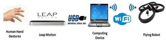
Fig.2: Connection between system components
