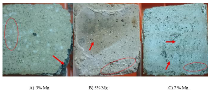
Figure 4) Specimens immersed in magnesium sulfate solutions of A) 3% Mg, B) 5% Mg, and C) 7% Mg after 6 months after drying for 5 days in room temperature.
