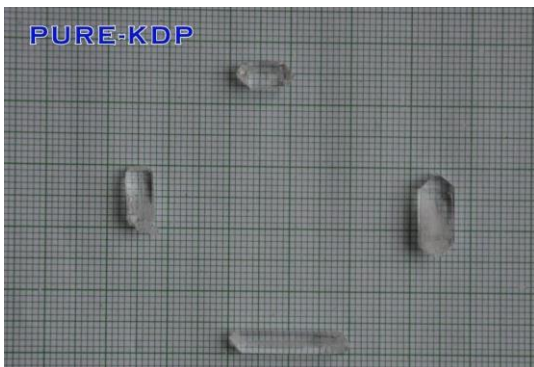
Pure KDP crystal grown from gel
