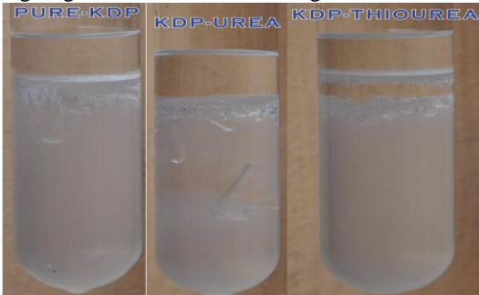
Figure.1.1: Pure, urea and thiourea doped KDP crystals near the interface and inside the gel.
