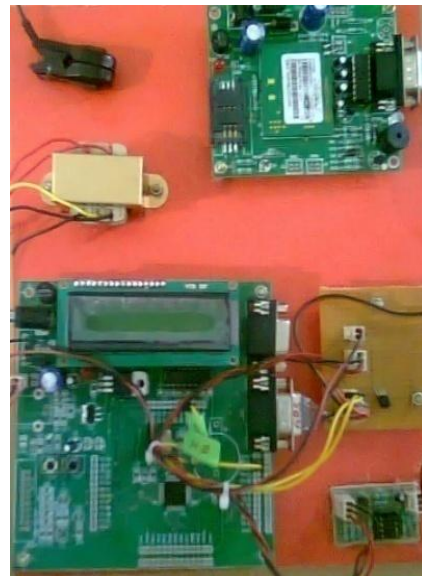
Fig7. Complete circuit to read heartbeat and temperature
