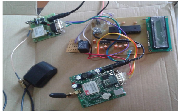
Fig. 2. GT-FAST vehicle module
