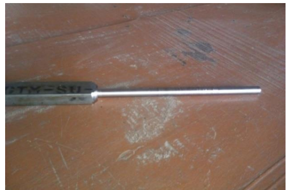
Figure.3: Inconel 718 rectangular bar machined to round bar
