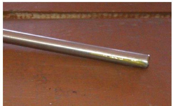
Figure.4: Bright extruded bar of SS 304
