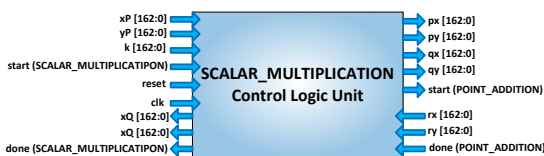
Figure 8: Scalar Multiplication Control Logic Unit
