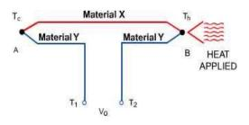
In a typical temperature measurement application, thermocouple A is used as a "reference" and is maintained at a relatively cool temperature of Tc. Thermocouple B is used to measure the temperature of interest (Th) which, in this example, is higher than temperature Tc. With heat applied to thermocouple B, a voltage will appear across terminals Tl and T2. This voltage (Vo), known as the Seebeck emf, can be expressed as: Vo = axy x (Th - Tc)
