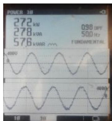
7.9 b Voltage and Current waveforms Under AHF ON condition,
