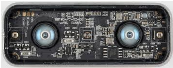
Figure 2. Leap motion teardown
