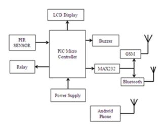
Fig1.Security System Block Diagram
