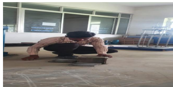
Fig 5.3 Demoulding of cubes
