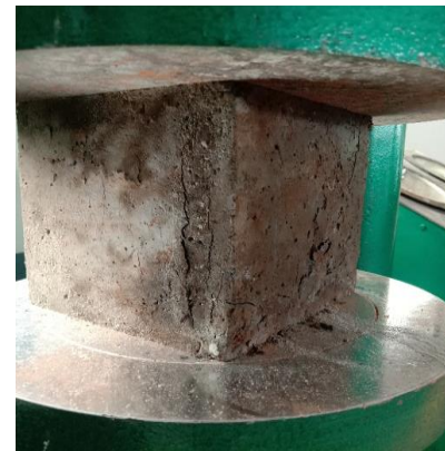
Fig. 2 Failure of cube
