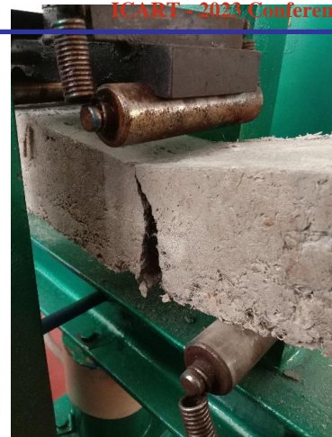
Fig.6 Failure of beam
