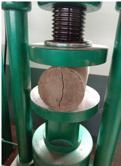
Fig. 4 Failure of cylinder
