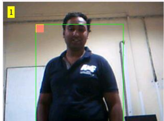
Figure 1: boundingbox as green color,red is the color tag as an identity mark.
