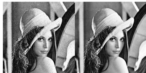
Figure 1. Sample Lena image with 5% random noise and denoised picture.
