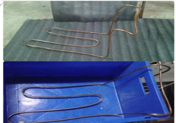
Figure 4. Heat Exchanger setup
