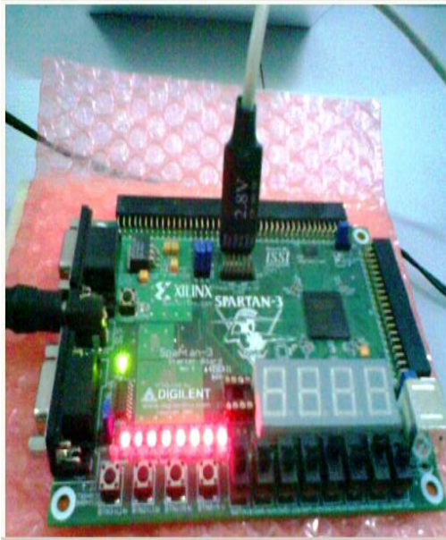
Fig.13. Lab Set-Up for Implementation of Conventional Controller for Maintaining Cane Level
