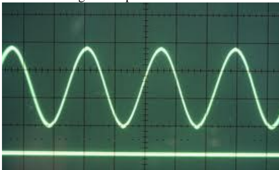
Fig.22 Sine wave on CRO through FPGA Spartan3E
