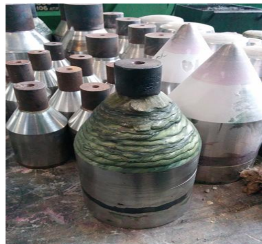
Fig 2 Disk coated with stellite 6.
