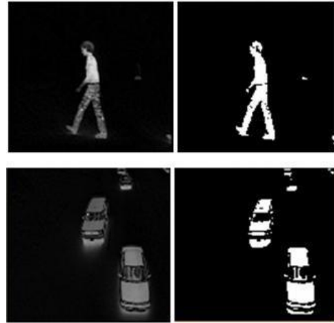
Fig.10 FPGA output shown using VB interface for background subtracted image and threshold applied image.
