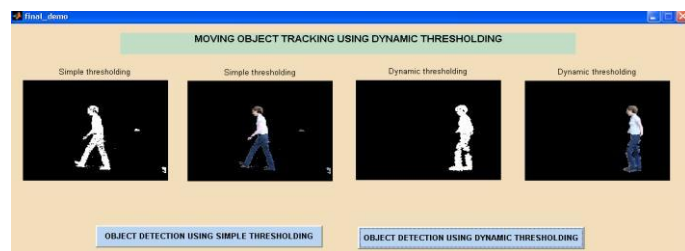
Fig.7 Matlab simulation results for simple and dynamic threshold shown in binary and color image formats.
