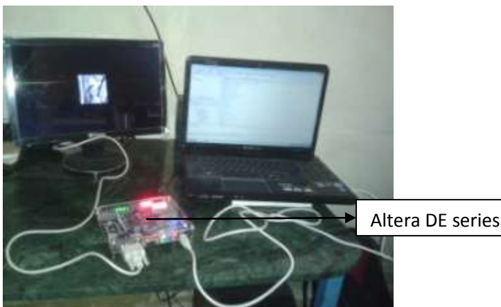
Figure 2. Experimental Setup of Altera for image display in monitor
