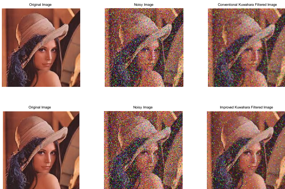
Fig2: Pictorial results for Conventional and Improved Kuwahara Filter on color Lena image (Noise Density =0.3)
