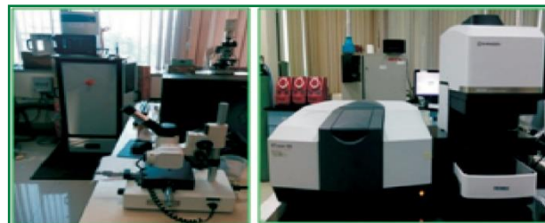
Figure-4: Four ball Tester (Ducom) & FTIR Instrument with Microscope (Shimadzu)
