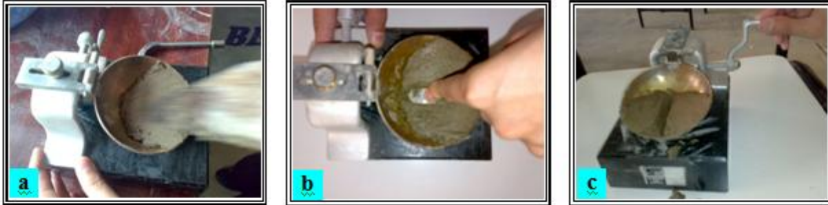
Figure (2) Stages for performing the liquid limit test
