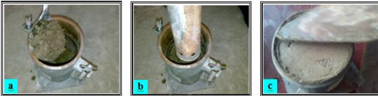
Figure (3): Steps for achievement the compaction test.
