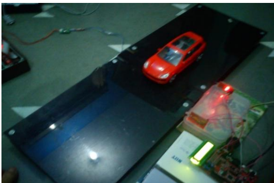
Figure 4 : WIM prototype; IR sensor sensing the vehicle
