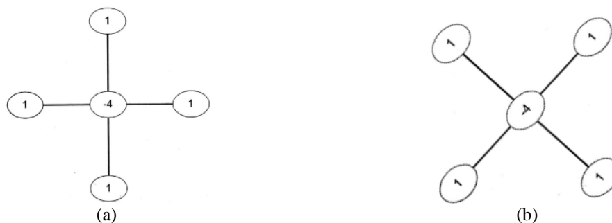
Figure 2: Stencils of 5-point formula for (a) full-sweep and (b) half-sweep iteration, respectively.
