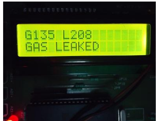
Fig. 7. Gas leakage is Monitoring on LCD display
