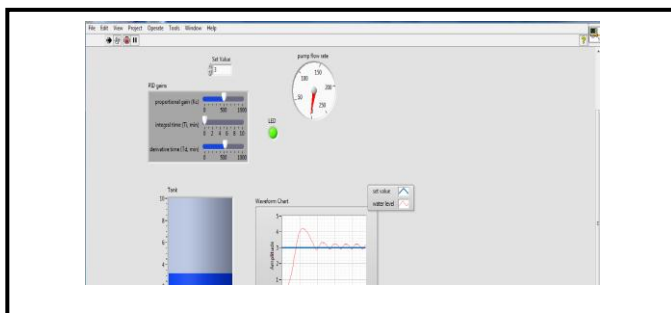
Fig 4.3. Front Panel of water level controller
