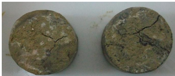
Figure 7. Example of the formation of cracks during wetting.
