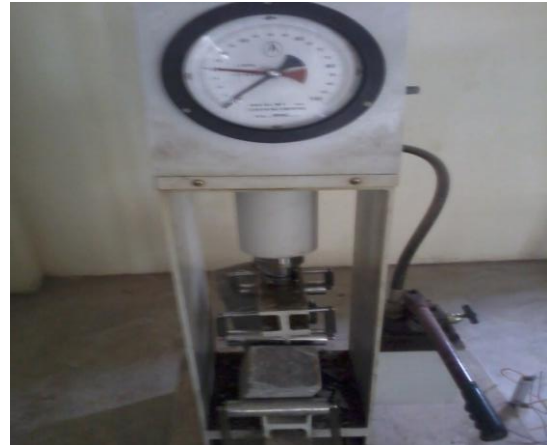
Figure 5: Determination of Flexural strength of Prism
