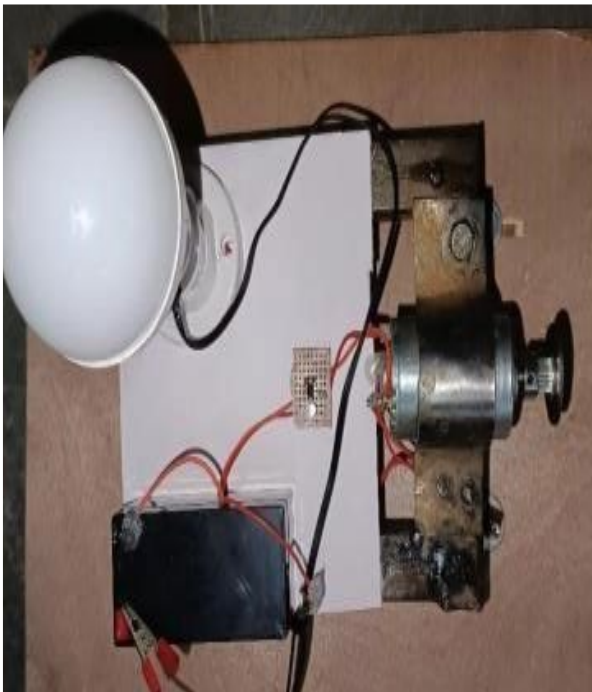
Figure 3:Battery,generator &amp; load system
