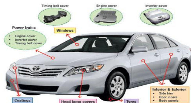
Figure. 2: Illustration of the usage of polymer nanocomposites parts.
