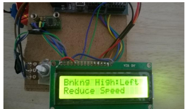
Figure 6.7 Display when vehicle is negotiating a curve
