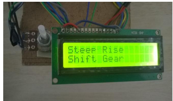
Figure 6.5 Display when vehicle is negotiating the steep rise
