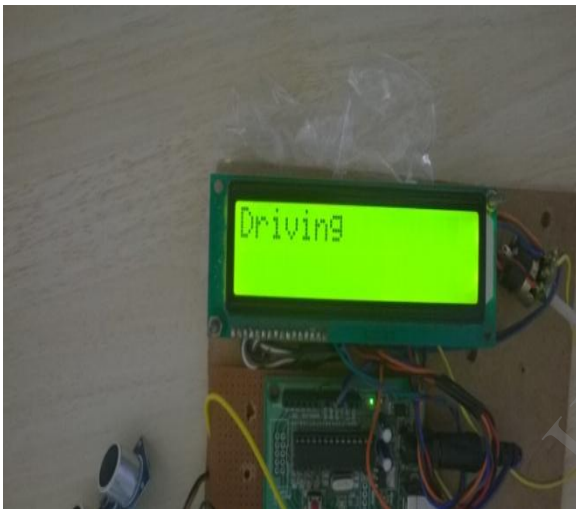
Figure 6.2 Display when automobile is in driving state with no obstacle
