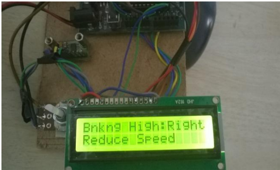
Figure 6.8 Display when vehicle is negotiating a curve
