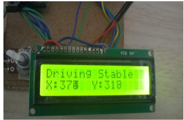
Figure 6.4 Display when vehicle is moving in stable state
