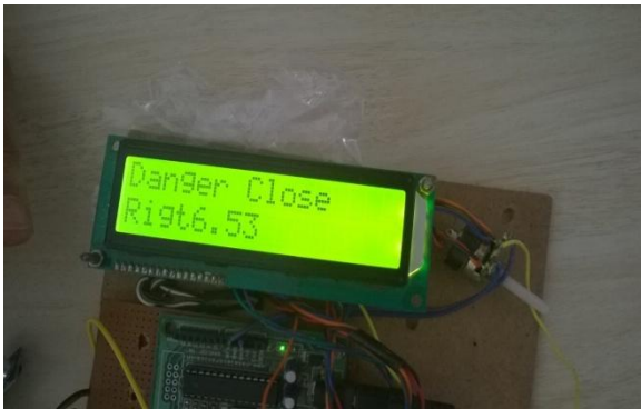
Figure 6.3 Display when the right sensor detects obstacles
