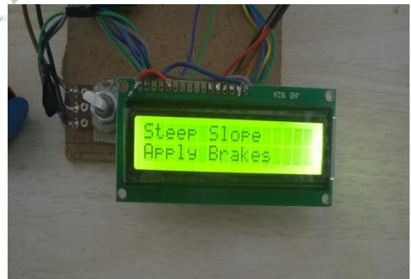
Figure 6.6 Display when vehicle is driving through the slope
