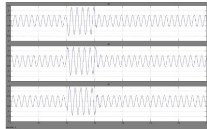
Fig. (5) Differential current signals of 3 phases in over-excitation condition
