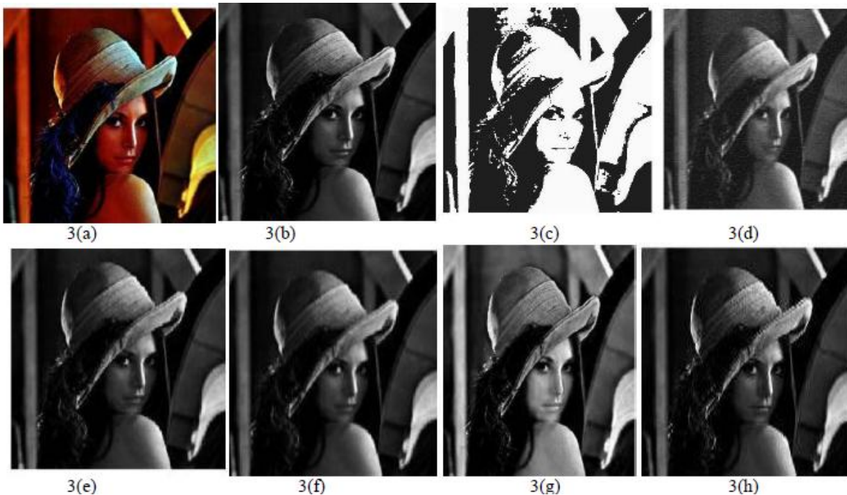
Fig 3: Lenna.jpg (a)original image, (b)grayscale image, enhanced image with (c)Thresholding, (d)Gaussian filter, (e)Spatial Lowpass filter,(f) spatial avg filter, (g) Fuzzy Adaptive filter (h) Proposed fuzzy technique.
