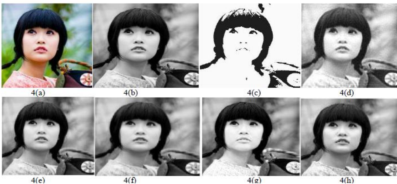
Fig 4: Girl.jpg (a)original image, (b)grayscale image, enhanced image with (c)Thresholding, (d)Gaussian filter, (e)Spatial Lowpass filter,(f) spatial avg filter, (g) Fuzzy Adaptive filter (h) Proposed fuzzy technique.
