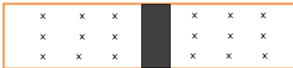
Figure 3. Schematic representation of Butt welded joint with the locations of hardness testing
