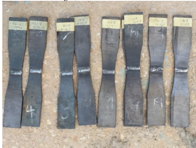
Figure (2) specimens welded using SMAW process
