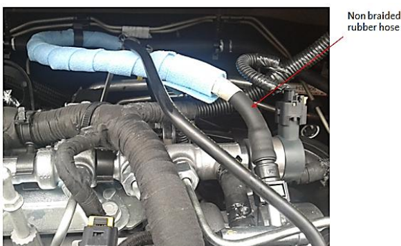
Figure 9. Non-Braided Rubber Hose as Fuel Return Line
