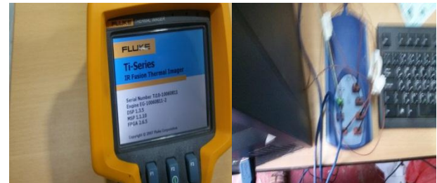
Fig. 3. (a) Infrared Thermal camera (b) Temperature Data logger
