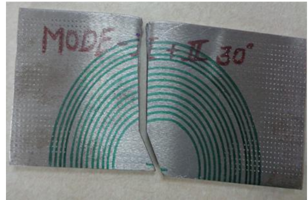
Fig.:- (b) For Mixed Mode-I+II, 30° after failure
