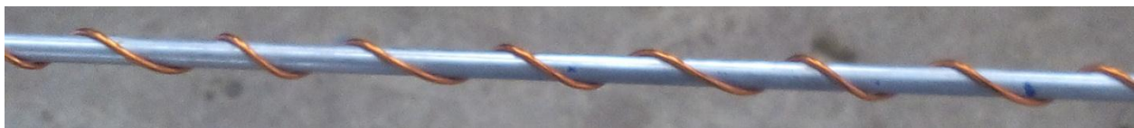
Fig.1. Helical coiled insert ( p/d ratio = 2).
