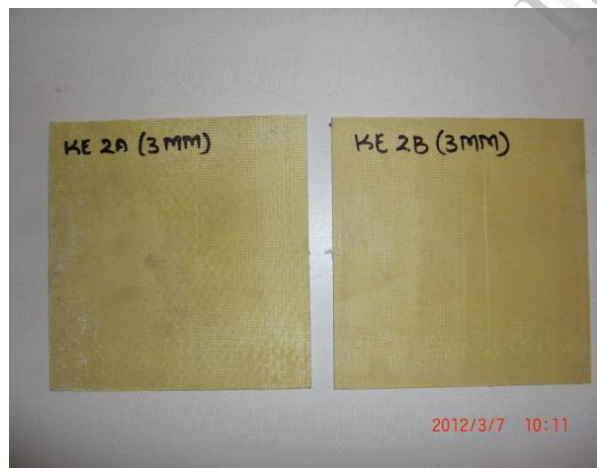
Fig 5.2: Machined Impact Test Specimens as per ASTM (D 3763) Standards
