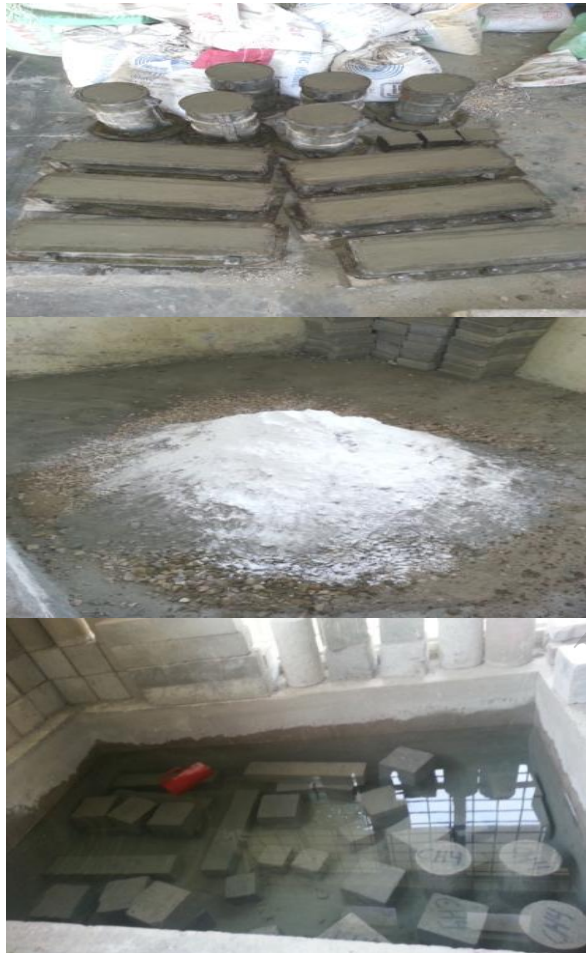
Fig. No.-1:- Casting and Curing Of Specimens
